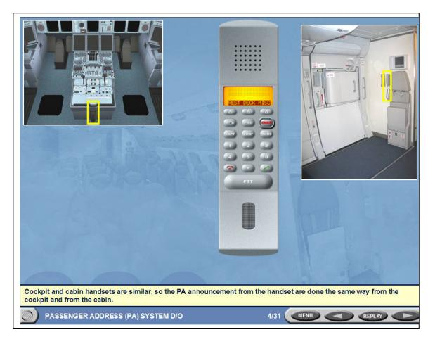
CAPTION: Passenger address handsets are installed in all large passenger aircraft. A dedicated handset is fitted in the cockpit for the use of the pilots and at a cabin-crew station. Illustrated here is the Airbus 380 system, similar to the one installed on the Boeing 767 and 757.
