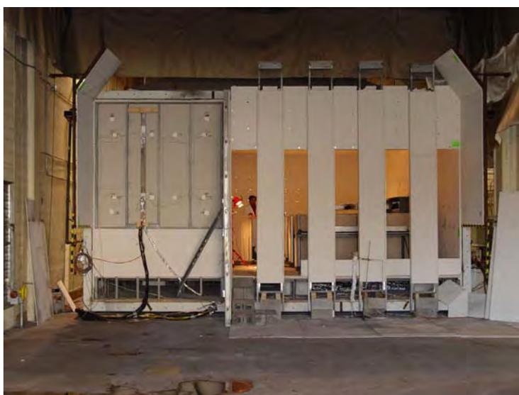
**Figure 3–6. NIST measured the thermal behavior of gypsum/steel wall assemblies subjected to severe fire conditions.**
