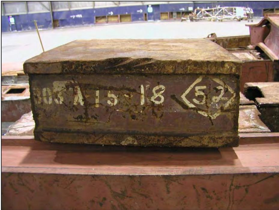
Figure F-6. (a) Characteristic stenciling found on the lower portions of the exterior column panels for sample C-14. (b) Characteristic stenciling found on an interior core column for sample B-6152.
