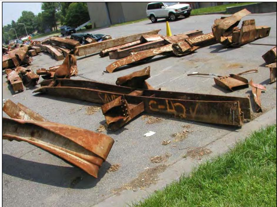
Figure 1–9. Other recovered wide flange sections, shown is sample C-42.
