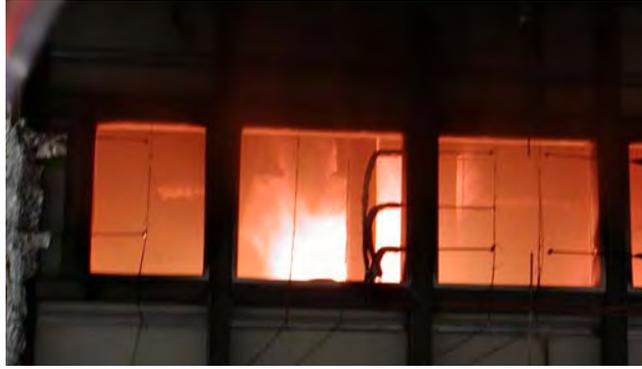
**Figure 3–3. View of fire compartment from air exhaust outlet several minutes after the start of a fire test. Note: the flame impingement on the steel trusses and bar.**
