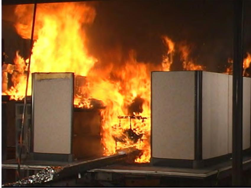
Figure J-17. Photograph of workstation near the peak heat release rate in test 2.
