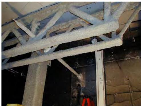
**Figure 3–2. Insulated steel trusses, steel rod and steel column inside the NIST large-scale fire laboratory.**
