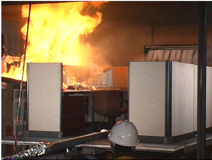
**Figure J-16. Photograph of workstation soon after ignition in test 2.**
